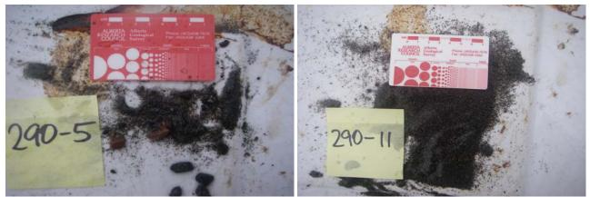
Figure : Medium and coarse sand interlaced with small 0.5cm to 1cm rounded gravel sampled in the area south of Tree Island. These sediments are considered to be suitable for eulachon spawning.
