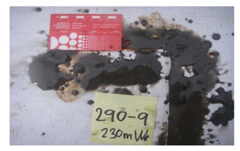
Figure : Fine sand with mud clasts and releasing organic-rich gas sampled from the area east of Tree Island between log booms. This sediment type is considered too fine for eulachon spawning and will due to the release of organic-rich and likely egg toxic gases represent an environment that is unsuitable for eulachon egg deposition.
