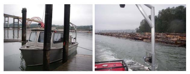
Figure : Terra Remote Sensing Inc. research vessel that is used as the operating platform for seismic profiling docked on the left photograph and operating the boomer system (center bottom of picture) on the right photograph.
