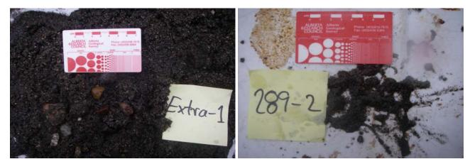
Figure : Coarse sand with rounded pebbles and 100% medium to coarse sand sampled from the area north of Douglas Island in the mouth of the Pitt River. These sediments are considered to be suitable for eulachon spawning.
