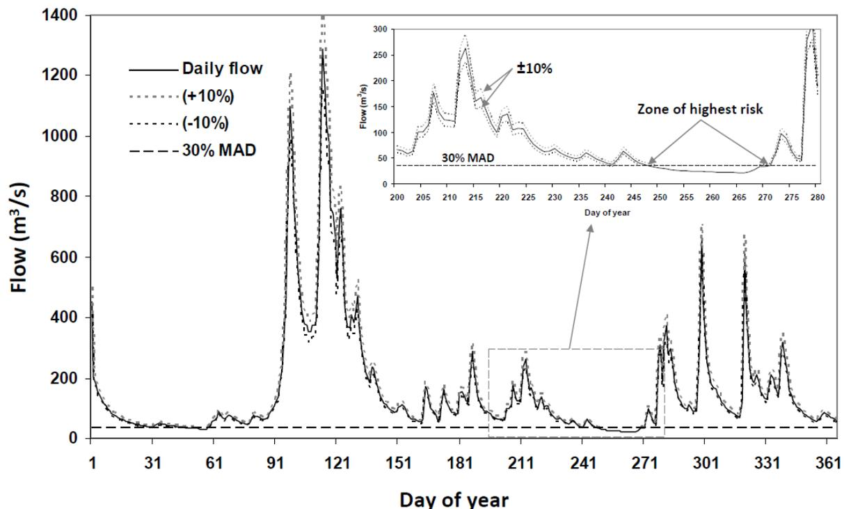
Figure 2: Graphic depiction of  $\pm 10\%$  instantaneous flow and of 30% Mean Annual Discharge (MAD). Refer to Figure 3 for detailed examination of zone of highest risk. - (Courtesy of D. Caissie, 2012)
